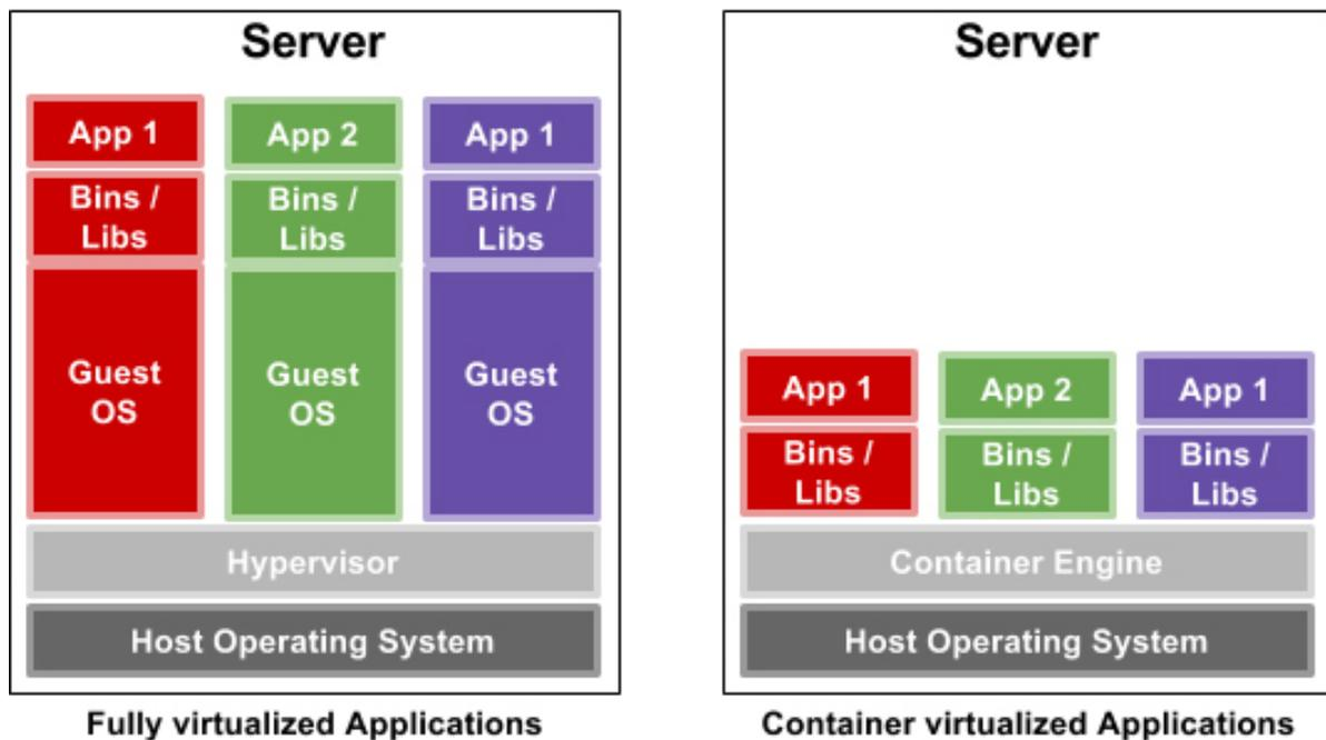
**FIGURE 1. A Comparison of Traditional Virtualization to Containers**
