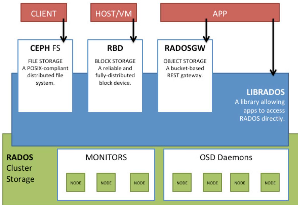
**FIGURE 1. SUSE Enterprise Storage Architecture**
