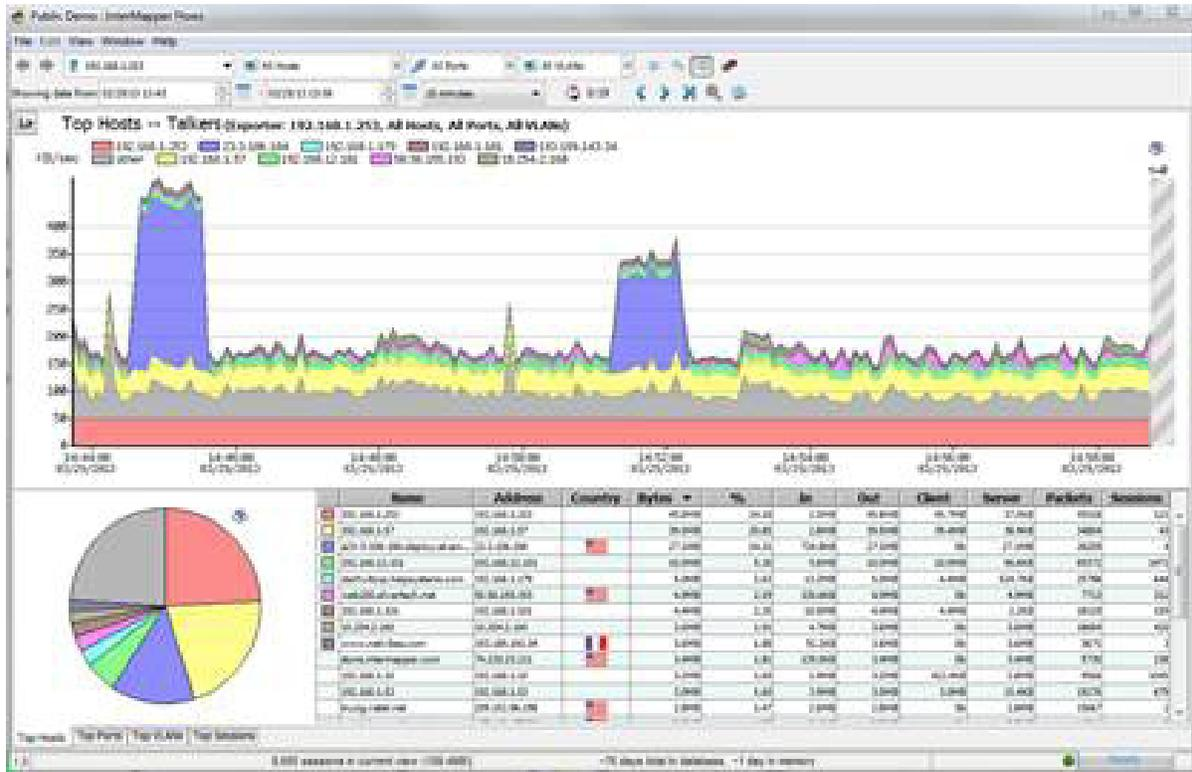
**FIGURE 2.** Netflow sensors allow the network monitoring staff to examine the amount and type of traffic flowing on the network.
